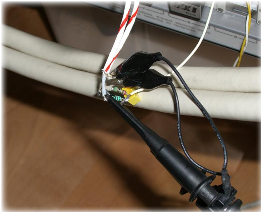
The two ECL lines connected to -2 V_{CC} via 50 Ohm pulldowns and to the scope probes.
